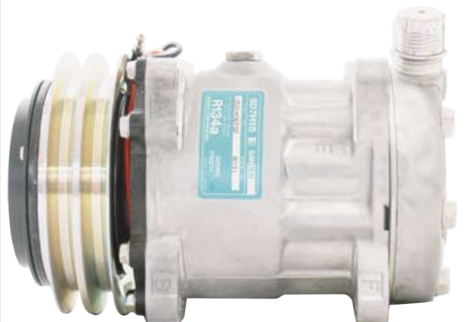
Baxters Part #: ACM8031 • Compressor to suit Sanden 12V SD7H15 Fittings: Vertical Standard o'Ring Application: Universal Rubber Damper Pulley Dia: 132 No. of Grooves: 2GA
