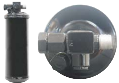
Baxters Part #: ADR1045 Size: Height 255mm Diameter 76mm Application: Kenworth
