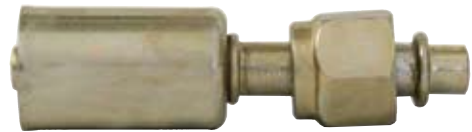
STEEL BEADLOCK FITTING Baxters Part #: AFS1303 Fitting Size: #10 Description: Female O'ring Straight Hose: #10 Thread: 7/8"-14
