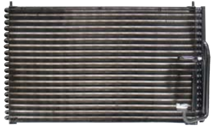
Baxters Part #: ACN1001 Dimensions: 660 x 386 x 38mm Application: Falcon EF/EL 10/95 - 8/96
