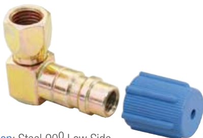
STEEL BEADLOCK FITTING Baxters Part #: AFS1322 Fitting Size: #8 Description: Female O'ring 90° Hose: #8 Thread: 3/4"-16
