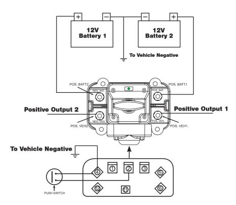
NOTE For Push Switch : Switch and Wiring must be capable of handling 50A Peak
